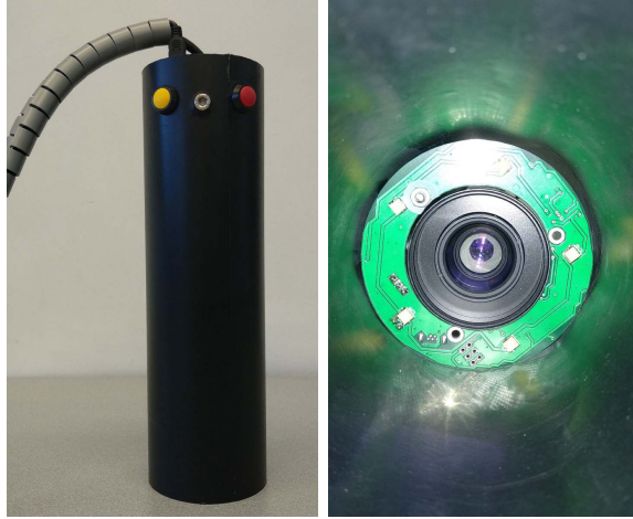
Figure 4.3: Acquisition setup: light field camera housing (left) and the camera main lens plus the illumination LED ring (right).
